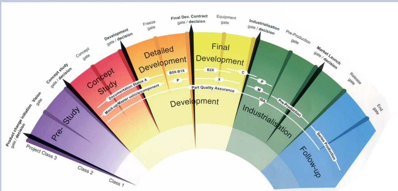
**Fig. 2.** The Volvo Corporation has developed a 'Global Development Process' GDP, which describes development processes with regard to new products and production systems. The built-in check-points, 'gates', cannot be passed until all demands at the previous level have been met. Volvo Powertrain in Skövde, in the light of the described research project, has begun to integrate ergonomics and working environment in the GDP.
