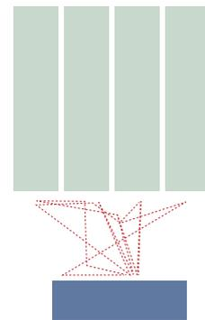
**Fig. 7.** Alternative material exposure after Japanese model with narrower and deeper frontages gives shorter walking-time, in this example 16 m per cycle, less load carrying, and less losses in value-adding time.
