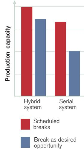
**Fig. 5.** Ergonomics in simulated flows. A comparison of production systems when a 'break as desired opportunity' is introduced.
