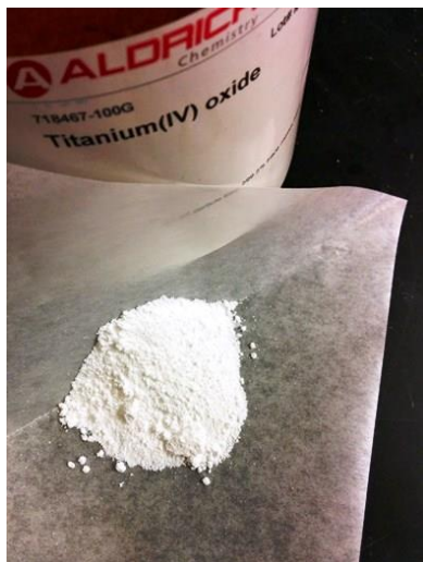
Figure 3: Titanium dioxide nanopowder. Particle size is roughly 21nm according to the manufacturer.
