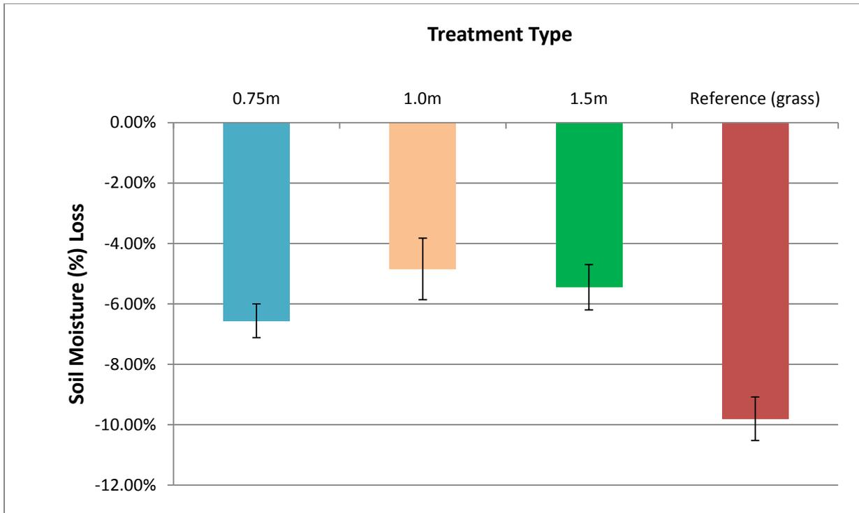
**Figure 3.6: Average soil moisture (%) loss over a 21 day drought from July 1-21, 2011 for each treatment type with standard error**
