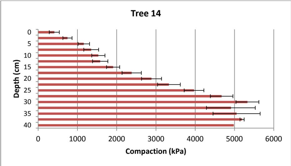
Average soil compaction (kPa) (0-45 cm in depth) for reference plots without grass
