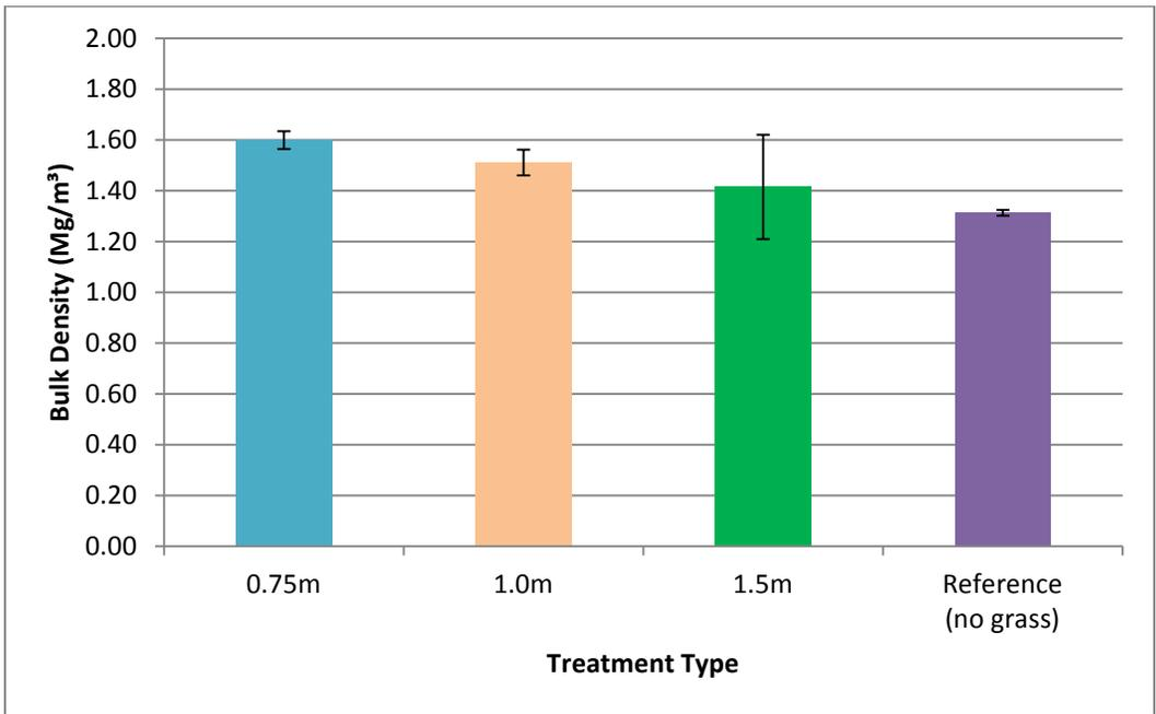
Average bulk density (Mg/m<sup>3</sup>) for each treatment type with standard error
