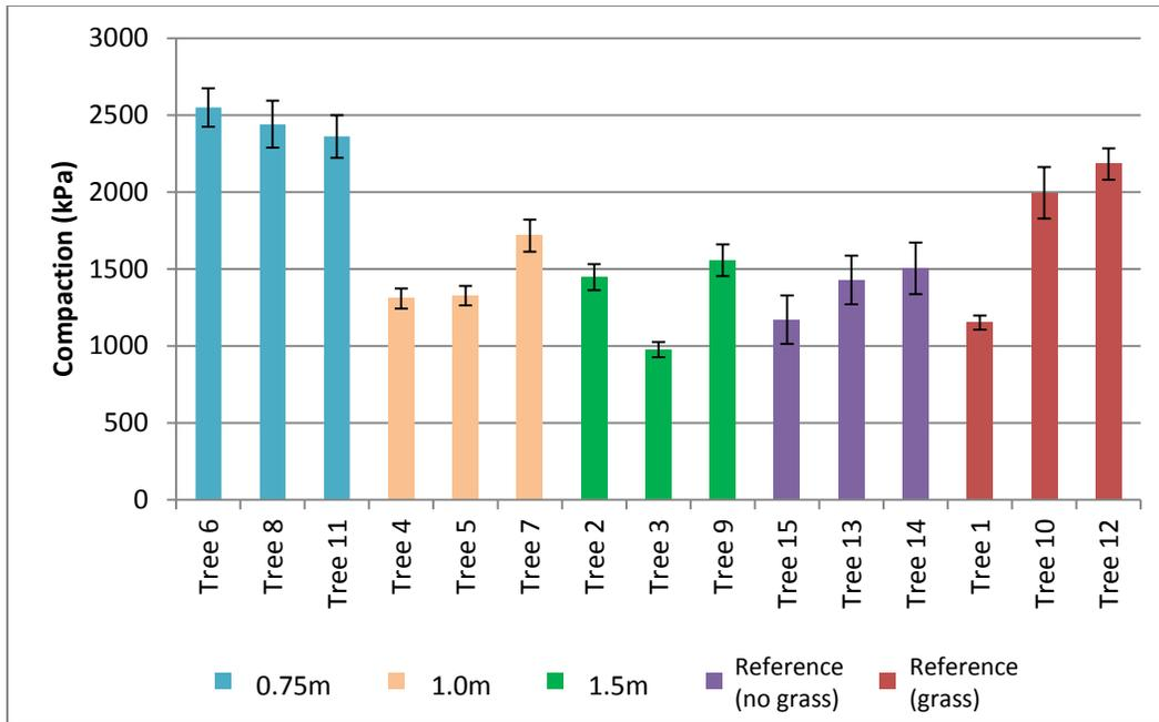
Average soil compaction (kPa) (0-20 cm in depth) for each tree with standard error
