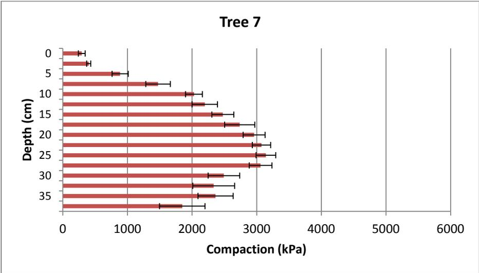
Average soil compaction (kPa) (0-45 cm in depth) for 1.0 m treatment plots
