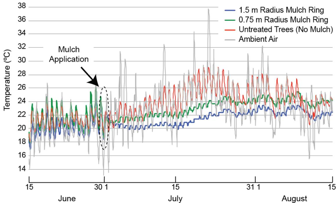
**Figure 3.7: Temperature (°C) comparison between mulched and non-mulched trees during the period of June 15 to August 15, 2011**
