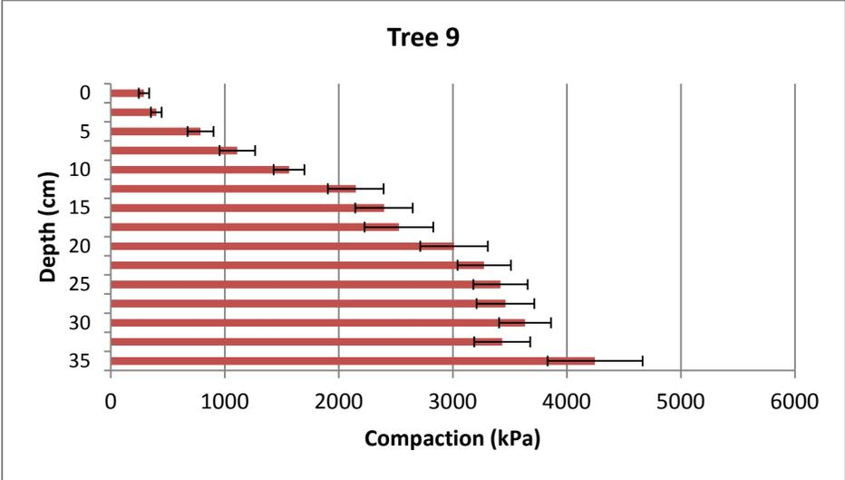
Average soil compaction (kPa) (0-45 cm in depth) for 1.5 m treatment plots
