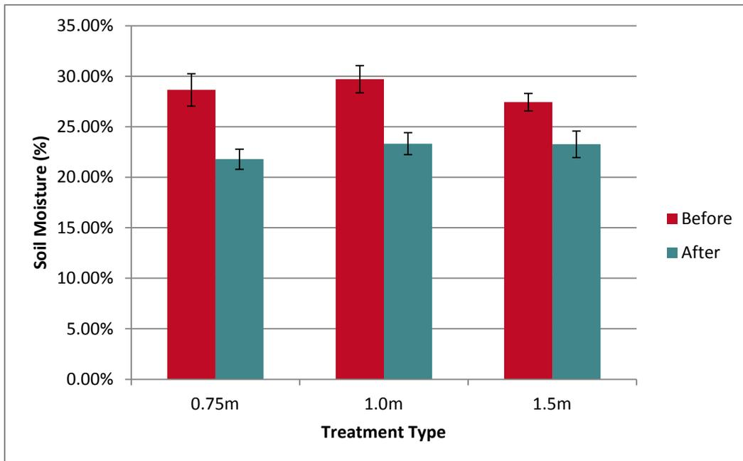
Average soil moisture (%) before and after mulch application for each treatment type with standard error
