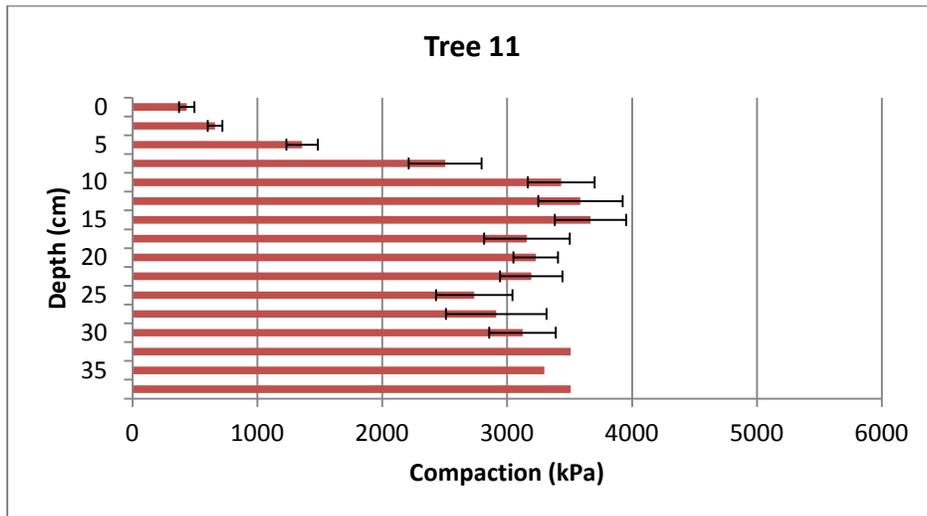
Average soil compaction (kPa) (0-45 cm in depth) for 0.75 m treatment plots
