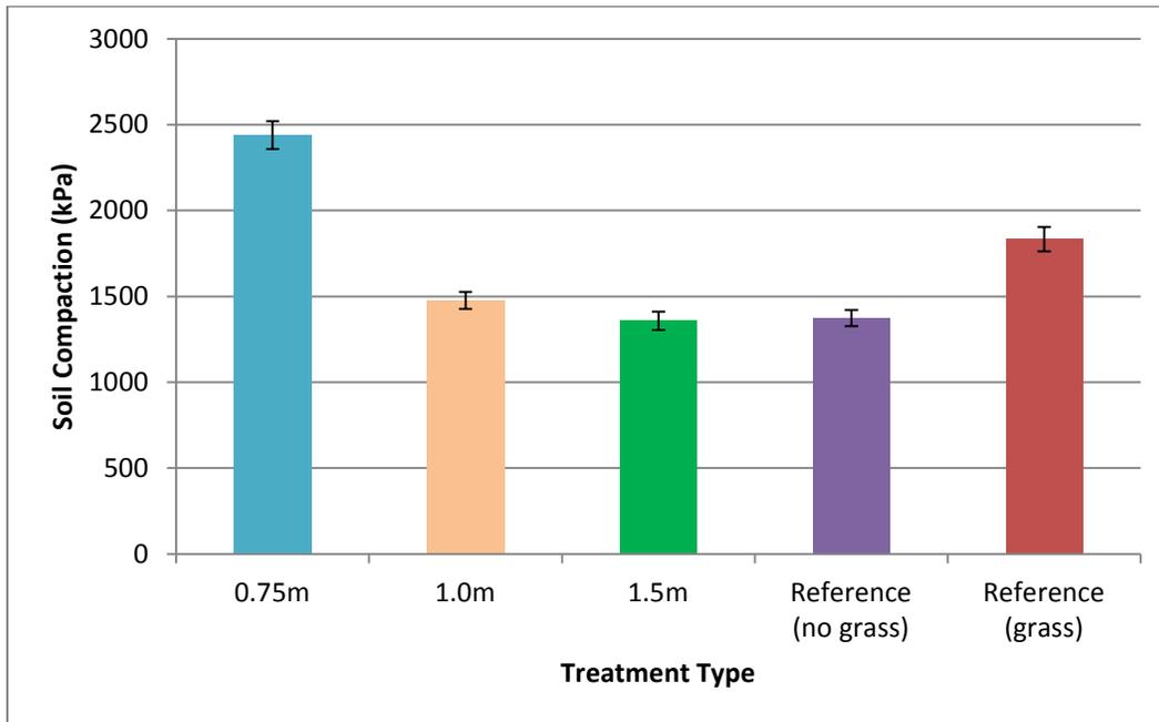
Average soil compaction (kPa) (0-20 cm in depth) for each treatment type with standard error
