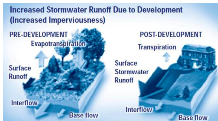
Figure 2: Illustration of effect of development on stormwater
