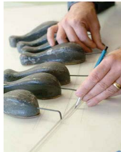
Figure 3.2.1.3 - Shipbuilder's spline tool: An example of how simple tools can inform complex systems and languages
