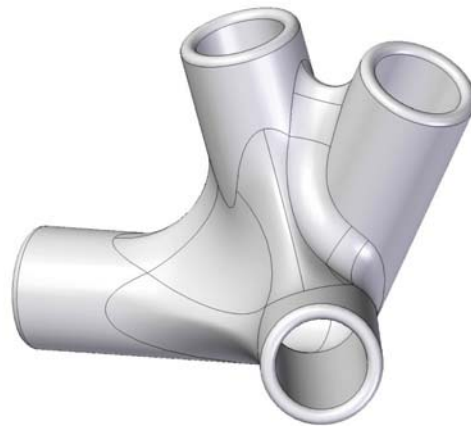
Figure 3.4.1.5 - Component structural refinement to increase integrity prior to print
