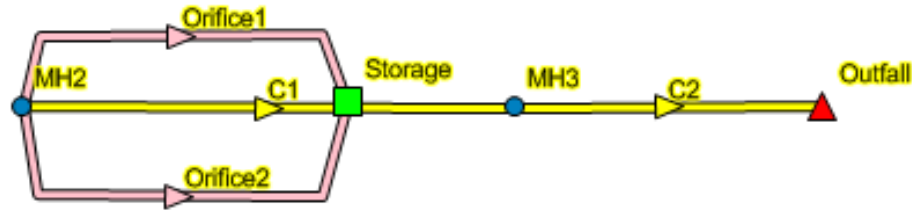
Figure 8 Representation of Orifice-Storage system in SWMM
