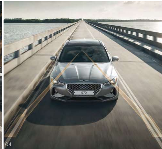
04. Lane Keep Assist _ Drift outside your lane without signaling and the Lane Keep Assist 9 system first warns you with haptic vibrations through the steering wheel, as well as audible and visual cues. If the vehicle continues to approach the edge of its current lane, Lane Keep Assist can provide steering assistance to bring the vehicle back on course.
