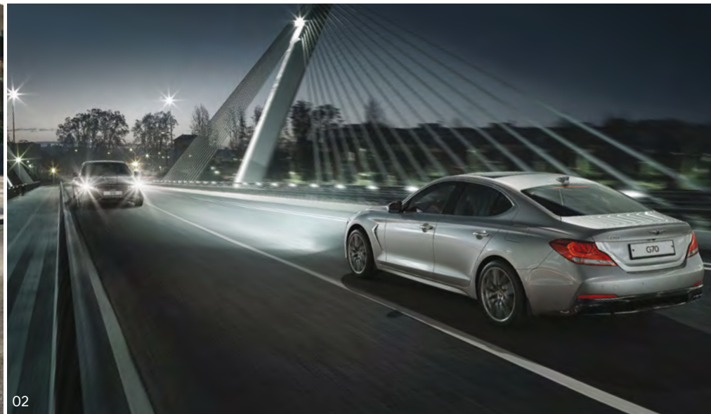
02. High Beam Assist _ Using the front-mounted camera and light detection technology, High Beam Assist automatically switches between high beams and low beams when traffic is detected ahead.
