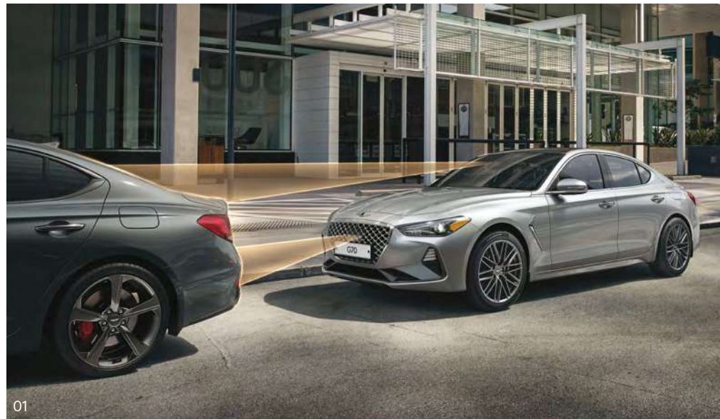
01. Forward Collision Avoidance-Assist (FCA-A) _ Forward Collision Avoidance-Assist 7 uses a forward camera and radar sensors to detect rapidly closing distance between your vehicle and the vehicle ahead. If a potential forward collision is detected, warning notifications alert the driver. The system can provide full braking assistance to help avoid an imminent collision at speeds between 8 and 75 kilometres per hour for vehicles or 8 and 65 kilometres per hour for pedestrians.
