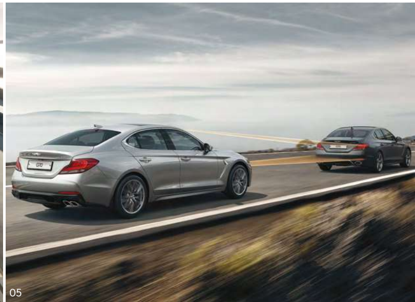
05. Adaptive Cruise Control _ Adaptive Cruise Control 10 with stop-and-go capability adjusts your preset speed and distance from the vehicle ahead. It will even come to a full stop and then start again, without driver input, when the vehicle has been stopped for less than three seconds.
