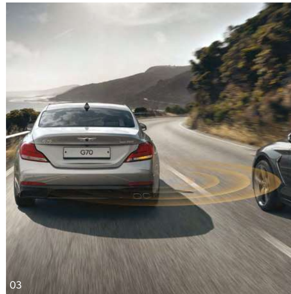
03. Blind Spot Collision Warning _ The Blind Spot Collision Warning 8 system heightens awareness by alerting the driver when there is a vehicle in their blind spot, or rapidly approaching, as they attempt to change lanes. In models equipped with the optional Head-Up Display, warnings are even projected onto the windshield for unparalleled situational awareness.
