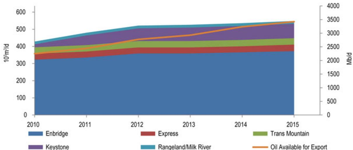
Figure 2: WCSB pipeline takeaway capacity and supply available for export (orange line) up to 2015 (Government of Canada, 2017).
