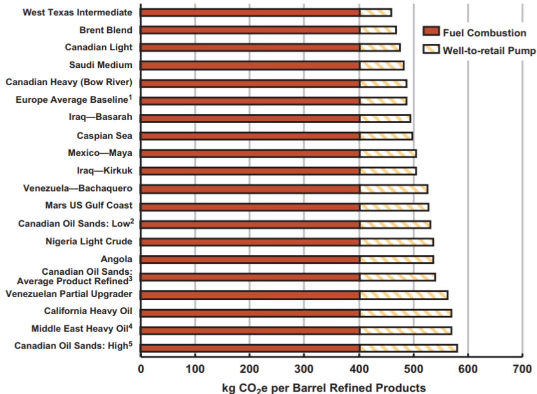
Figure 7: Well to wheels greenhouse gas emissions for oil sands and other crudes (IHS CERA, 2011).
