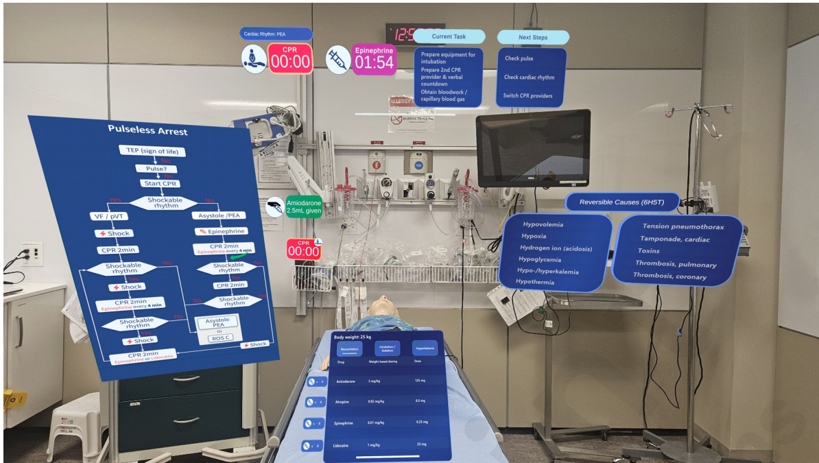
Figure 2. Team leader display showcasing real-time CPR and medication timers, visual alerts for task progression, and stepwise guidance for current and upcoming guideline tasks during a simulated CA scenario.
