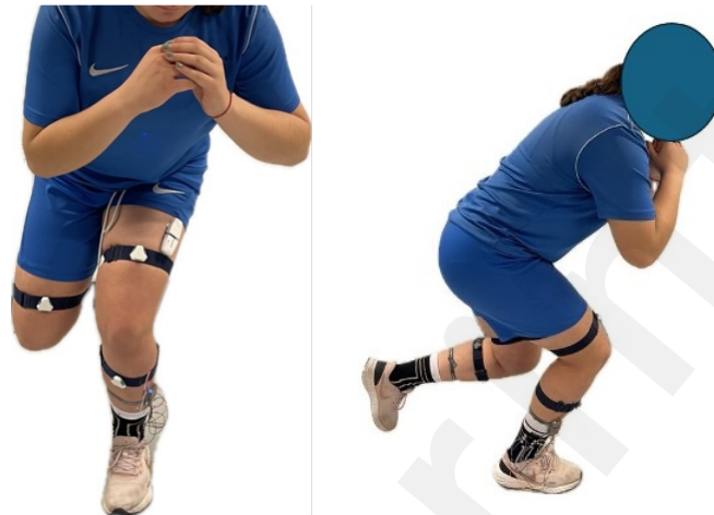
Figure 1. Study participants interacting with the DAid® smart sock system, the PLUX Wireless Biosignals (muscleBAN kit) wireless electromyography device, and the NOTCH® inertial sensor system.
