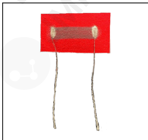
Figure 1. Motion Tape sample with conductive wire leads given to the physical therapists for evaluation.
