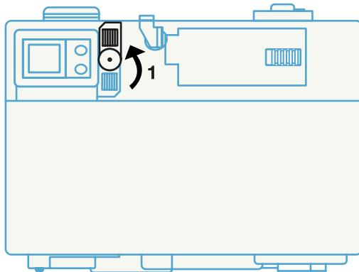
Unfold the rewind crank (2) and rotate it clockwise (in the direction of the arrow) until the resistance from pulling the film disappears. Fold up the rewind crank again and flip down the rewind tab (1). Open the back cover as previously instructed (**p.4**) and remove the film cartridge.
