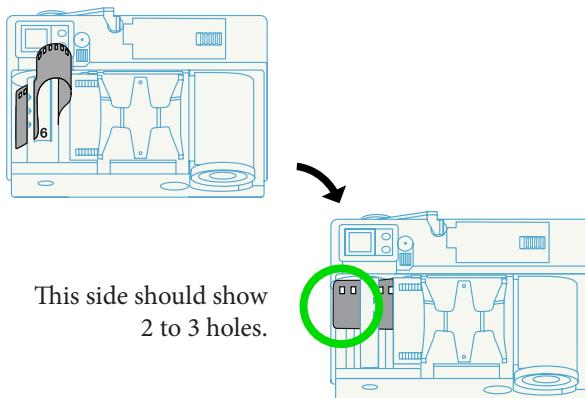
Don't close the back yet. Turn on the camera and press the shutter release button (7) firmly all the way down. Pull the winding lever (8) **all the way** to its stop.
