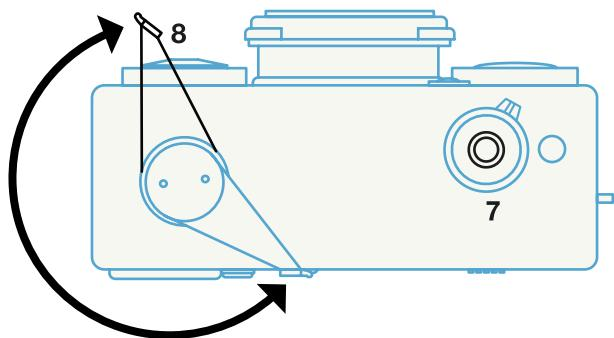
Please make sure the advance lever has been rotated **as far as it can go**, as shown in the illustration below, until the tip of the lever is **pointing forward**.
